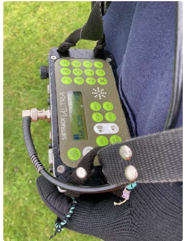
The receiver showing the frequency, the volume and the accuracy.
